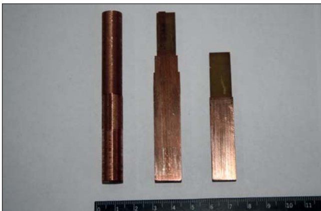
The view of HEC Cu-W billets fabricated at 900°C at intensity of compression 5 GPa.
